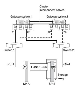
You improve availability by having one connection from each adapter on each gateway in the HA pair. Then, if one path from a gateway node fails, the other path from the node is used; failover in the gateway HA pair does not occur.
